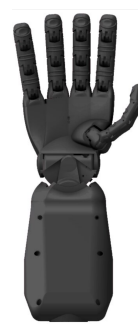
(a) RH8D Adult Size Dexterous Robot Hand de Seed Robotics.
