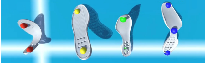
Figure 1: Shoe soles deformation utilizing NVIDIA Flex Unity’s library. Spheres represent grasping points.
