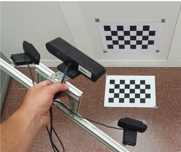
Figure 4: Camera rig recording plane data from the floor and a wall equipped with one checkerboard each
