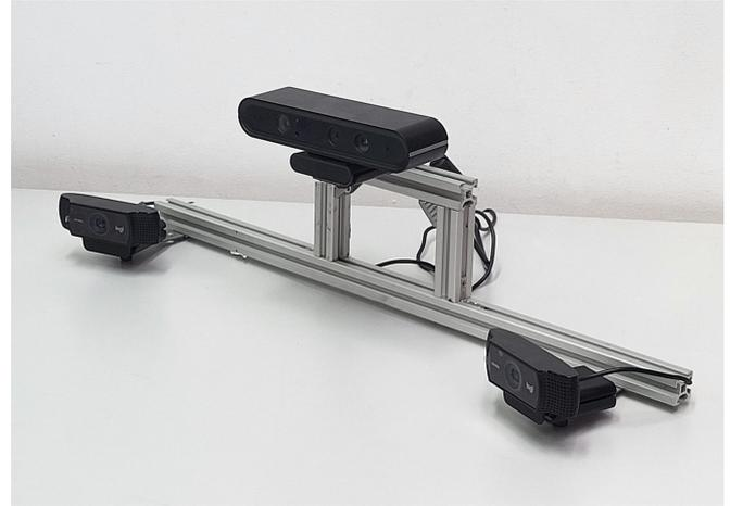
Figure 2: Test setup used for the experiment: RGB-D device (Orbbec Astra) in the middle, two RGB sensors (Logitech C922 Pro) left and right
